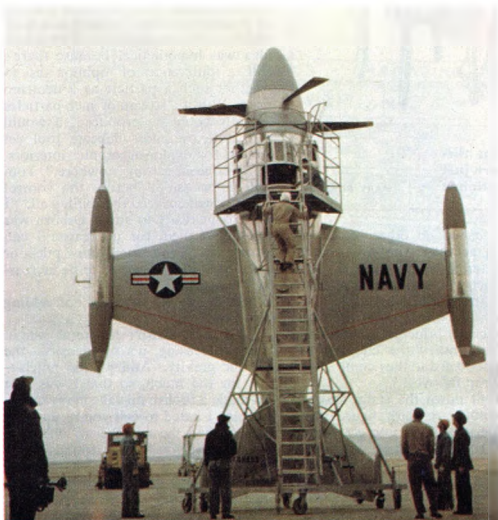
Pilot uses a 20-foot ladder to enter Lockheed's XFV-1 cockpit. For emergency landings, he also carries rope ladder in plane Collier's for April 2, 1954
