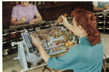
A Western Electric girl assembles one of the more than 300 "brain cells" that guide a Nike battery's missiles.
