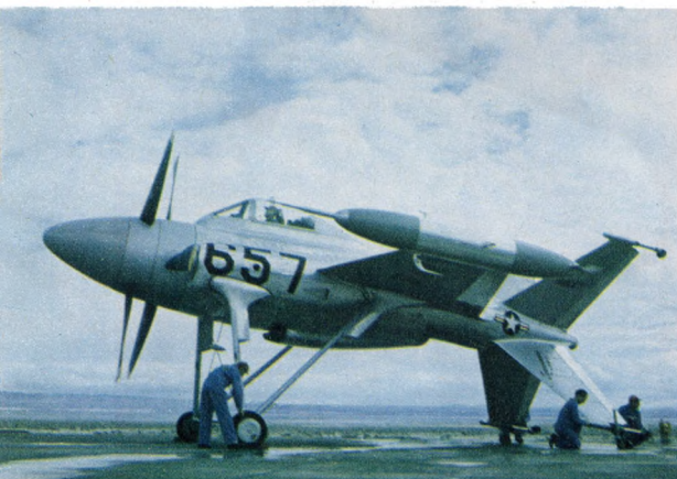
Old-style landing gear used in taxiing tests was made extra high to ensure that propellers would clear ground. Charles A. Lindbergh, who was shown the aircraft, said: "I haven't seen a landing gear like that on a plane for twenty years"
