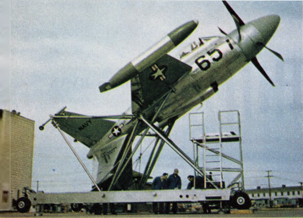
Both Convair and Lockheed designed massive cradles to move VTO planes from vertical to horizontal position for easier maintenance. Photo shows Lockheed's device in the process of lowering the XFV-1 during tests at Edwards Air Force Base
