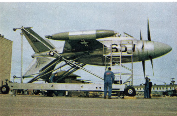
XFV-1 rests horizontally in cradle. Mechanics work on the aircraft from platform at right. Note the landing wheels attached to four tail vanes. For taxiing and level-flight tests, Lockheed devised temporary landing gear shown below
